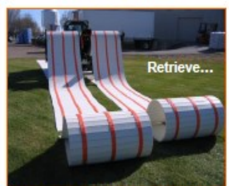
Connect Trax to Spools - Back up and Begin Roll up of Trax
